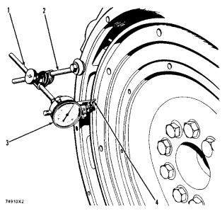
CHECKING BORE RUNOUT OF THE FLYWHEEL
