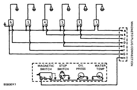
IGNITION SYSTEM DIAGRAM FOR SOLID STATE MAGNETO (FAIRBANKS MORSE) (3306 Engine)
