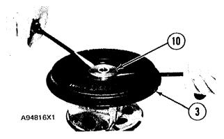
10. Use two screwdrivers to remove insert (10) from cartridge housing (3).
