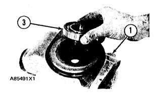
3. Install the shaft and bearing (3) in housing (1).
