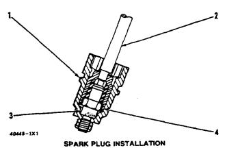
1. Adapter. 2. 3/8 In. Drive extension. 3. Spark plug. 4. 2P5481 Spark Plug Socket.
