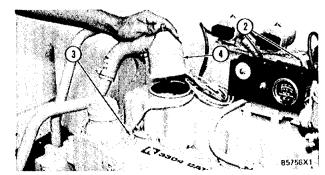
3. Connect wire (2) to the stop switch. Install water temperature sending unit (3) in the cylinder head.
