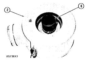
5. Remove tube assembly (6), arrestor and the Oring seal from body (2) as a unit.
