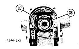
26. Use a press to remove bearing (38) from housing (36).
