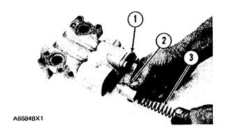
2. Install plunger (2) and spring (3) for the oil cooler bypass valve.
