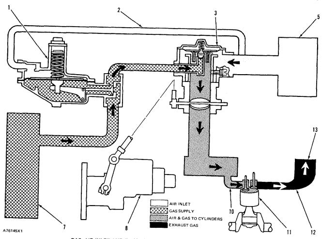
GAS, AIR INLET AND EXHAUST SYSTEM WITHOUT TURBOCHARGER (3304 and 3306 ENGINES)
