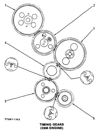
1. Drive gear for magneto. 2. Idler gear for magneto drive gear. 3. Camshaft gear. 4. Crankshaft gear. 5. Idler gear for oil pump. 6. Drive gear for oil pump.
