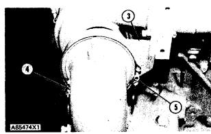
3. Remove bolts and nuts that hold support (3) to the exhaust manifold. Remove support and coupling (6).
