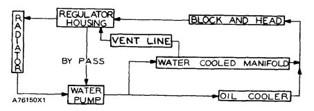
SCHEMATIC OF COOLING SYSTEM
