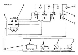
IGNITION SYSTEM DIAGRAM FOR SPARK GAP MAGNETO (3304 Engine)
