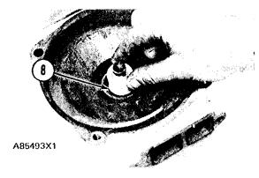
9. Remove the spring from the seal assembly (9). Use hand pressure and the tool (which is with the replacement ring) to install the seal assembly. Push seal assembly on the shaft until seal faces make light contact.
