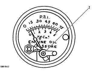
OIL PRESSURE GAUGE 2. Adjustment screw.
