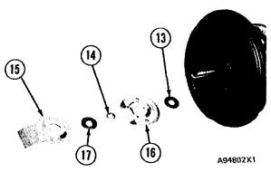
11. Install ring (13), bearing (16), sleeve (14), ring (17) and deflector (15) in the housing.
