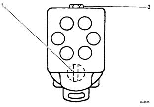
DRIVE TANG AND SLOT POSITION FOR 3306 ENGINE (Seen from Rear of Engine)
