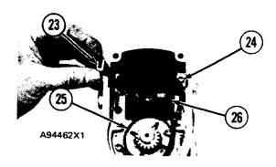
17. Loosen screws (24) and wedges (23) and turn rotor shaft assembly (25) until flux lock (magnetic field) is broken. Remove screws, wedges and coil (26) from the housing.
