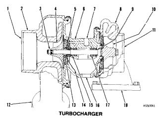
1. Air inlet. 2. Compressor housing. 3. Nut. 4. Compressor impeller. 5. Thrust bearing. 6. Center housing. 7. Lubrication inlet port. 8. Turbine housing. 9. Sleeve. 10. Turbine wheel. 11. Exhaust outlet. 12. Air outlet. 13. Sleeve. 14. Oil deflector. 15. Bearing. 16. Oil outlet port. 17. Bearing. 18. Exhaust inlet.
