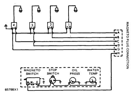
IGNITION SYSTEM DIAGRAM FOR SOLID STATE MAGNETO (FAIRBANKS MORSE)
