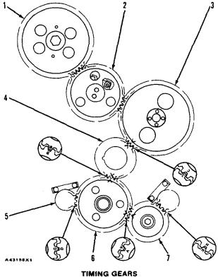
(3304 ENGINE) (2304 ENGINE) (2. Idle gear for magneto. 2. Idle
