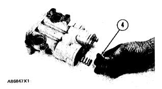
3. Install gasket, cover (4), washers and bolts for the oil cooler bypass valve.
