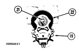
16. Use a press to remove distributor gear and shaft assembly (22) from the bearing support.
