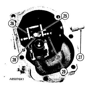
14. Remove lever (26) and shaft (27) from the housing.
