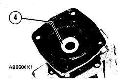
3. Put the ceramic ring (4) in position in the rubber seal. Use a cover for protection to install the ceramic ring. Install the ceramic ring evenly with hand pressure.
