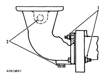
Put 5P3931 Anti-Seize Compound on threads of all nuts, bolts, studs and plugs (2).
