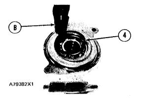
4. Install snap ring (4) in the housing with tool (B).
