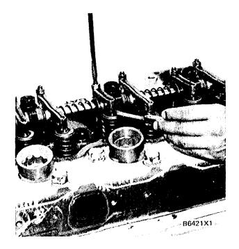
6. Install bracket (4) and the bolts which hold it to the cylinder head.
