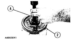
2. Use tool (A) to install the bearing in idler gear (2).
