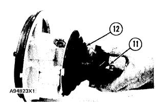
10. Install turbine shaft (11) in the cartridge housing.
