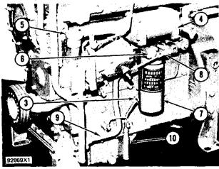
LUBRICATION SYSTEM COMPONENTS (3304 Engine)
