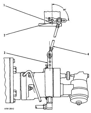
ADJUSTMENT OF LINKAGE TO THE CARBURETOR (Naturally Aspirated Engine Illustrated)
