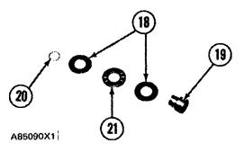
10. Put races (18) and bearing (21) in position on sleeve (19). Install ring (20) that holds the races and bearing on the sleeve.
