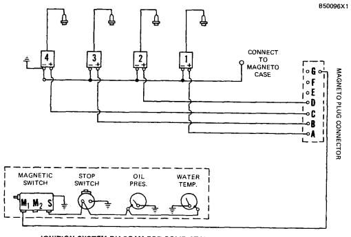
IGNITION SYSTEM DIAGRAM FOR SOLID STATE MAGNETO (ALTRONIC)
