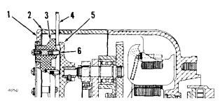
MAKING A CHECK OF THE BRUSH SPRING ADJUSTMENT
