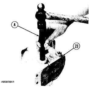
16. Remove plug and bearings (29) from housing (23) with tooling (A).
