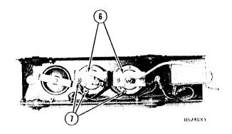
6. Remove brackets (6) that hold the gauges in position.
