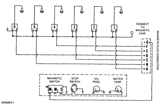
IGNITION SYSTEM DIAGRAM FOR SOLID STATE MAGNETO (ALTRONIC) (3306 Engine)
