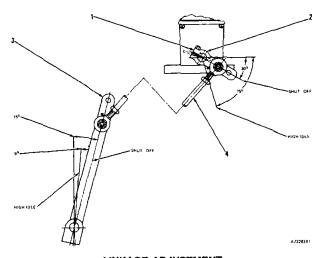
LINKAGE ADJUSTMENT (Naturally Aspirated Engine)
