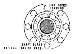
Discard the bearings if the races and balls or rollers are pitted, scored or burned. If the bearing is serviceable, coat it with oil and wrap it in clean paper. Do not unwrap new bearings until time of installation.
