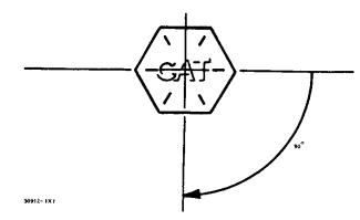
6. Put clean oil on the upper and lower halves of main bearings. Install the caps in their correct places. Install the bolts and washers. Tighten to 30 ± 3 lb.ft. (40 ± 4 N·m). Put marks on bolt heads and caps. Tighten each bolt 90° from the mark.
