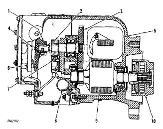
CROSS SECTION OF SPARK GAP MAGNETO
