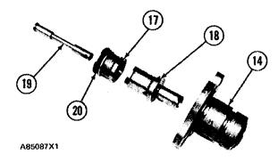
10. Remove O-ring seal (20) from sleeve (17).
