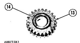
12. Inspect bearing (14) for wear and damage. Use tooling (A) to remove if necessary.
