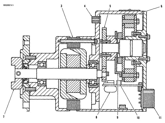
CROSS SECTION OF SOLID STATE MAGNETO (ALTRONIC)
