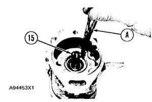
14. Use tool (A) to install snap ring (15) that holds the rotor shaft assembly in position.
