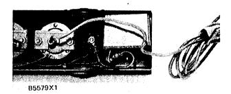
8. Remove gauges (8) from the instrument panel.
