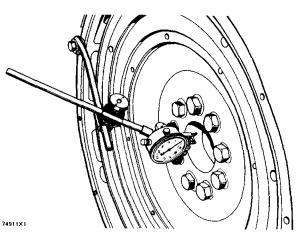
CHECKING FLYWHEEL CLUTCH PILOT BEARING BORE
