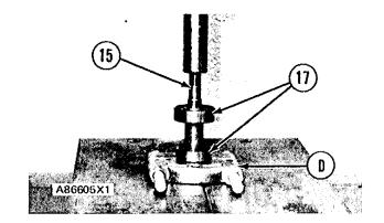
15. Remove ceramic ring (18) and seal.
