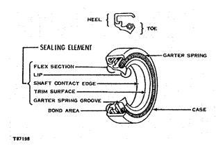
The main parts of a lip-type seal are the case, sealing element, and garter spring. The picture illustrates the construction of a simple lip-type seal. The cross sections show the terms "heel" and "toe" used to identify the sides of various types of seals.
