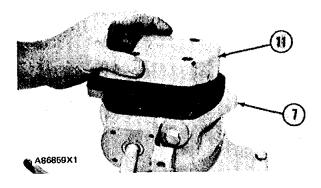
9. Install gasket and cover (11) on housing (7).
