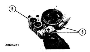
4. Put 5P3413 Pipe Sealant on the threads of the five plugs (6) and install plugs in oil filter base (5).
