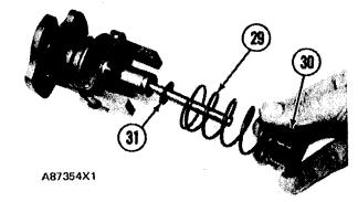
17. Put spring (29) and seat (30) in position on the weight assembly. end by:
