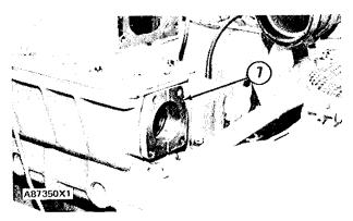
10. Remove adapter (11) and gasket from the after-cooler cover.
