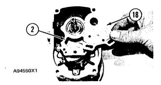
17. Install plate (18) on bearing support (2).
