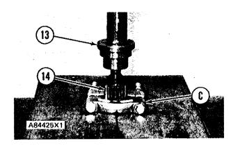
12. Install taper pin (15) that holds gear (14) in place. Move the metal (peen) on the small diameter end of taper pin (15) to hold the taper pin in place.
