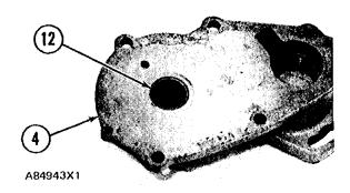
10. Turn adapter assembly (4) over. Inspect bearing (12) for wear and damage. If a replacement is necessary, bearing (12) must be destroyed to be removed.
