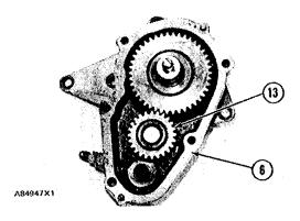
11. Remove idler gear (13) from housing (6).
