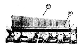
12. Remove aftercooler core (14) and gasket.
