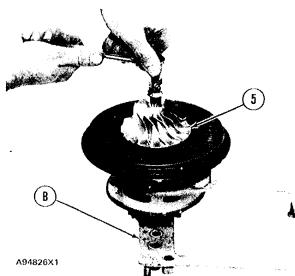
7. Remove turbine wheel assembly (7) and shroud (6) from the cartridge housing.
