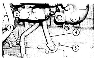
3. Remove bolt (3) and clip (2) from the inlet tube.
