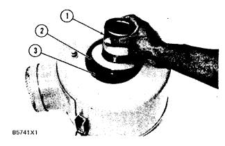
2. Install tube assembly (1) and arrestor (3) in the body.
