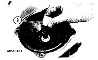
10. Install spring (10) on the seal assembly.
