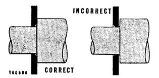
When pressing bearings into a retainer or bore, apply pressure to the outer race. If the bearing is pressed on the shaft, apply pressure on the inner race.
