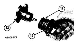
9. Put weight assembly (16) in position on cylinder (13). Install lockring (17) that holds the weight assembly on the cylinder.
