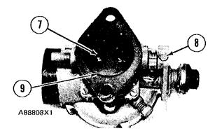
5. Remove throttle lever (8), lever stop and shaft as a unit.
