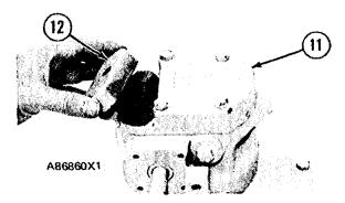
10. Put cover (12) and the gasket in position over the high idle screw and fasten to cover (11).
