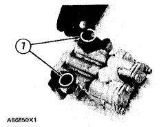
5. Put O-ring seals (7) in position on the oil filter base. end by:
