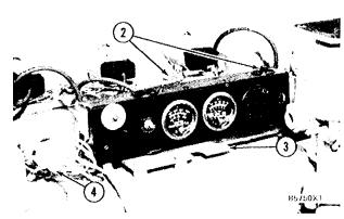
4. Disconnect oil pressure sensing line (5) and the wire that is connected to the bottom of the instrument panel. Remove the instrument panel.
