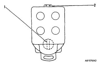
DRIVE TANG AND SLOT POSITION FOR 3304 ENGINE (Seen from Rear of Engine)
