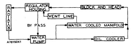
SCHEMATIC OF COOLING SYSTEM
