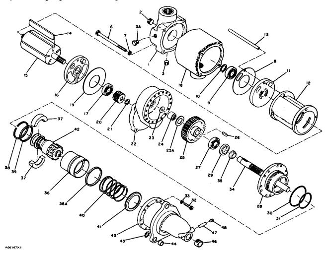
COMPONENTS OF THE AIR STARTER (INGERSOLL-RAND, SIZE 150 BMP,MODEL C OR E)
