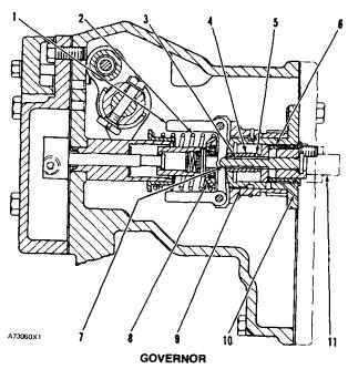
1. Governor weights. 2. Governor spring. 3. Valve. 4. Piston. 5. Oil passage. 6. Sleeve. 7. Oil outlet passage. 8. Spring seat. 9. Cylinder. 10. Oil inlet passage. 11. Governor shaft.
