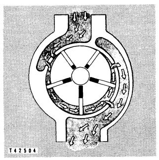
FLOW OF AIR THROUGH STARTING MOTOR (VIEWED FROM DRIVE END OF MOTOR)
