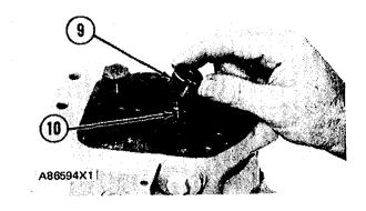
8. Install stop collar (9) on bolt (10) and fasten with the screw.
