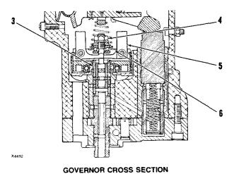
3. Pilot valve bushing. 4. Locknut. 5. Flyweight. 6. Spring seat.
