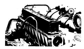
13. Remove eight bolts (16) and washers that hold the aftercooler housing (15) in place.
