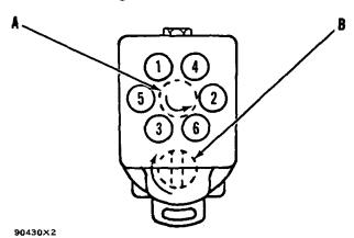
DIAGRAM OF MAGNETO NUMBERING (Seen from rear of engine)
