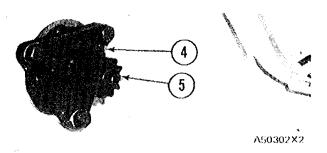
ENGINE TURNING TOOLS (Typical Example) 4.5P7306 Housing. 5.5P7305 Gear.
