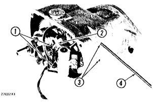
EDGE GAP ADJUSTMENT (Counterclockwise Magneto)
