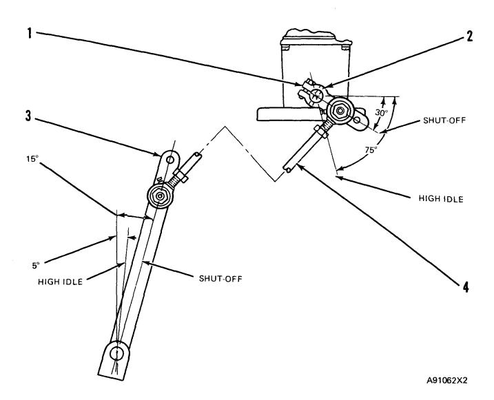
LINKAGE ADJUSTMENT (Naturally Aspirated Engine)
