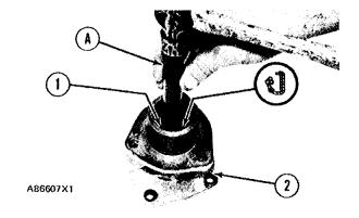
1. Install lip seal (1) in body (2) with tooling (A). Install lip seal even with bottom of bearing bore with the lip of the seal toward the bearings. Put a small layer of engine oil on the lip of the seal.
