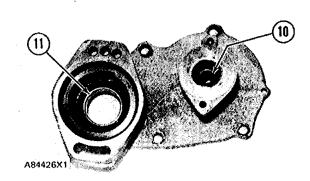
9. Inspect seal (10) for wear and damage. If a replacement is necessary, seal (10) must be destroyed to be removed.
