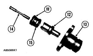
8. Install piston (12), sleeve (11) and valve (14) in cylinder (13).
