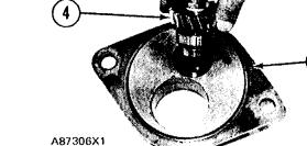
4. Remove shaft assembly (4) and bearings from housing (5).
