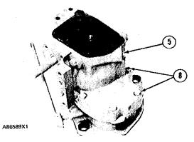
5. Remove bolts (8) that hold housing (5) in place. Remove housing (5) and gasket from the governor drive.
