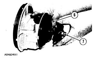
8. Remove seal ring (8) from turbine wheel shaft (7).
