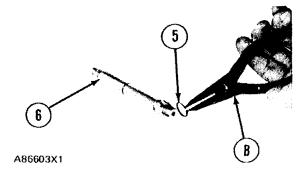
4. Install snap ring (5) on shaft (6) with tool (B).
