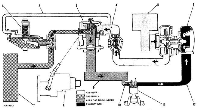
GAS, AIR INLET AND EXHAUST SYSTEM WITH TURBOCHARGER (3306 ENGINE)
