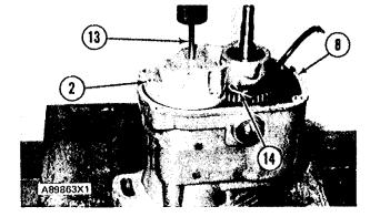
13. Install the three screws that hold bearing support (2) and clip (14) in position.
