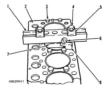
Install a .030 in. (0.76 mm) shim plus any added shims necessary to get the correct cylinder liner projection.
