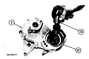
14. Put shaft (13) and gear into position in adapter.
