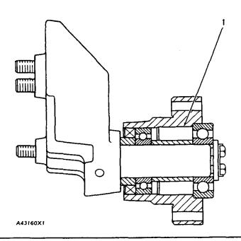
Fill chamber between bearings half full of 1P808 Grease before bolts are tightened.
