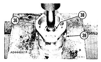
27. Remove vent cover (39) and screens from each side of housing (36).
