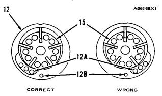
REAR VIEW OF THE CYLINDER AND ROTOR FOR CLOCKWISE ROTATION
