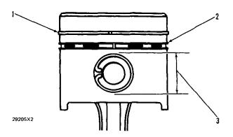
(3) Bore in piston for pin ..... 1.5011  $\pm$  .0002 in. (38.128  $\pm$  0.005 mm)
