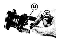
11. Put sleeve assembly (22) in position on valve (14). Make an alignment of the holes in the sleeve and valve.
