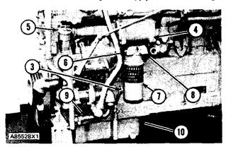
LUBRICATION SYSTEM COMPONENTS (3306 Engine)
