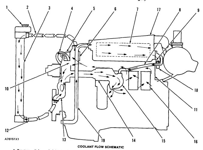
1. Pressure relief cap. 2. Inlet line for radiator. 3. Radiator. 4. Water cooled exhaust manifold inlet. 5. Vent line. 6. Temperature regulator. 7. Water cooled exhaust manifold. 8. Water cooled exhaust manifold outlet. 9. Cylinder head. 10. Internal passage. 11. Cylinder block. 12. Inlet line for water pump. 13. Water pump. 14. Oil cooler. 15. Oil cooler bonnet. 16. Cylinder liner. 17. Aftercooler. 18. Aftercooler outlet. 19. Inlet line from auxiliary water pump to aftercooler.
