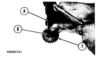
6. Put gear (7) in position over shaft (8) in housing (3).
