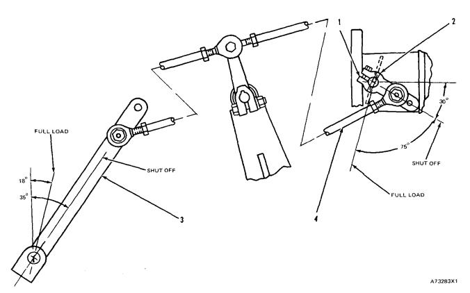
LINKAGE ADJUSTMENT (Turbocharged Engine)
