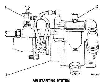
1. Starter control valve. 2. Oiler. 3. Air motor.
