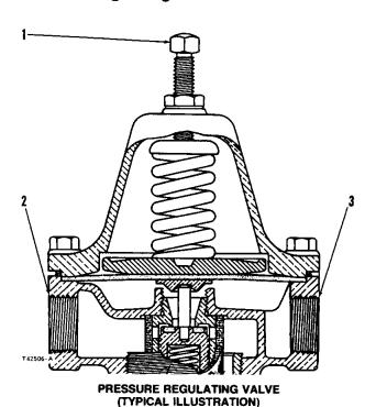
1. Adjustment screw. 2. Regulator inlet. 3. Regulator outlet.
