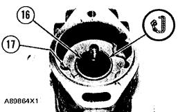
16. Install coupling pawl stop pin (17). Use the left hole as shown for counterclockwise rotation.
