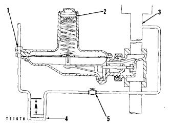
CHECKING LINE PRESSURE REGULATOR ADJUSTMENT (Schematic Diagram for Turbocharged Engine)
