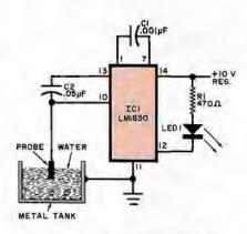
Fig. 3. Low-level detector flashes LED when probe in tank is exposed.
