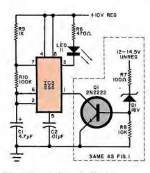
Fig. 2. Overvoltage indicator has a flash rate of 1.5 Hz.
