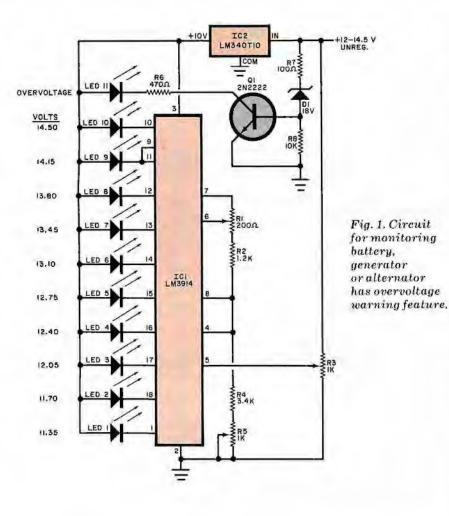
boat's electrical system is maintained at 10 volts by IC2. This potential was selected so that regulation occurs whether the boat's engine is running or stopped. The regulator can be used as the 10-volt source for all circuits described in this article. A GE-MOV V27ZA60 or similar suppressor can be installed between the
