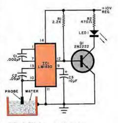
Fig. 6. High-water detector for grounded metal tank.
