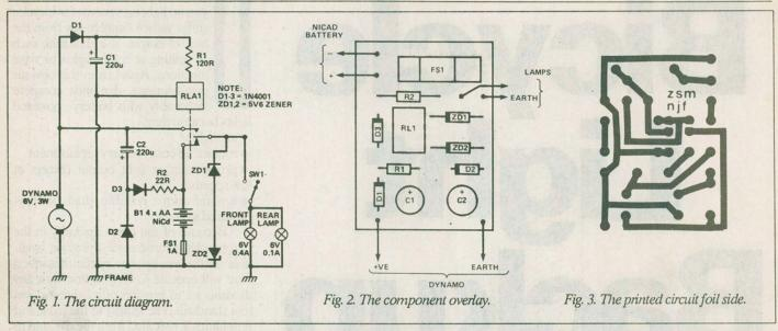
solidly connecting one terminal of the dynamo to the frame. Some commercial backup units require that the dynamo is isolated from the frame, easier said than done. The system described here does not impose such a restriction, thus making it easier to install by current and future dynamo users.
