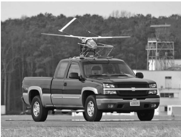
FIGURE 3.8 AAI Aerosonde vehicle-top launch cradle. (Copyright AAI Aerosonde a Textron Systems Company.)
