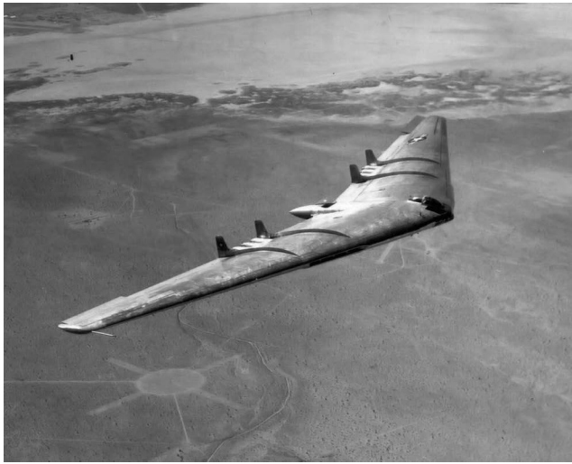
FIGURE 10.7 Northrop YB-49 flying wing (circa 1947-48). Note the vertical stabilizers necessitated by the lack of a flight dynamics computer. (U.S. Air Force image.)
