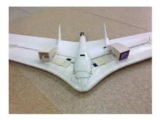
Fig. 16 The testing airframe - delta wing MAV
