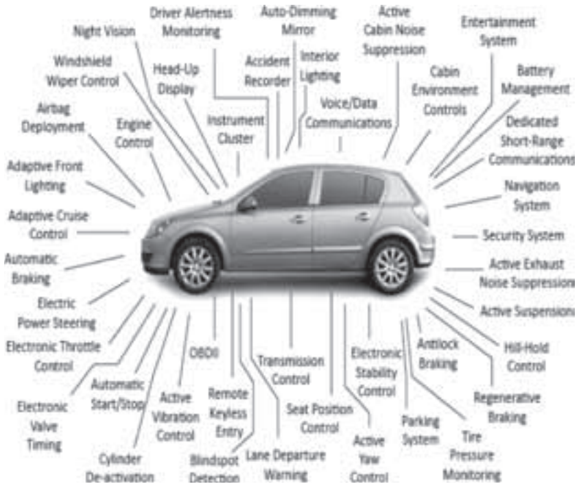
FIGURE 2-1 Types of electronics systems in modern automobiles. (Source: Clemson University Vehicular Electronics Laboratory.)
