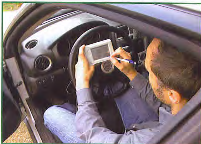
Figure 4. Subaru-programming with the handheld programmer from www.fastchip.nl
