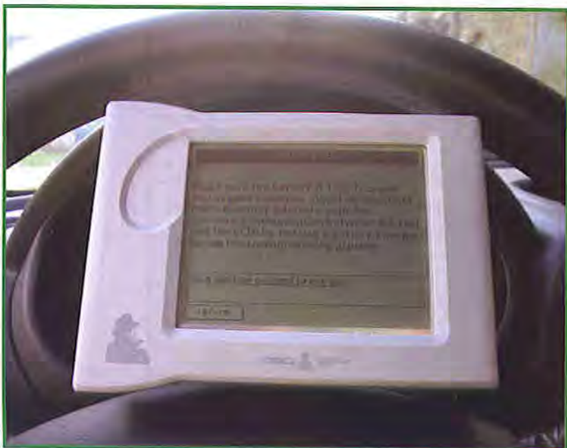
Figure 4. Subaru-programming with the handheld programmer from www.fastchip.nl
