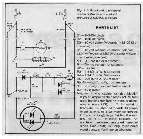
and diodes *D1* and *D2* make up a 0-to-6-volt dc voltmeter. When connected in series with 10-volt zener diode *D3*, this meter circuit becomes an expandedscale 10-to-16-volt dc voltmeter. Diode *D2* protects the meter against reverse polarity, while diode *DI* protects against overvoltage when the meter is connected in proper polarity.
