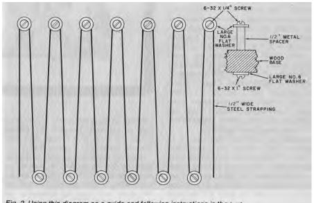
Fig. 2. Using this diagram as a guide and following instructions in the text, you can make up your own load resistor from 1/2-inch steel banding strap.
