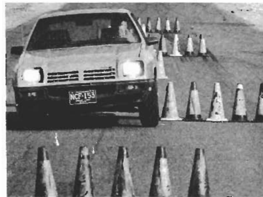
Low-speed slalom evaluates maneuverability. Spirit (top) displayed high body roll, was slowest. Nimble Champ (next to top) cornered much flatter, tied for win here, easily won high-speed lane-change. Surprising Chevette (next to bottom) tied Champ in slalom. Omni O24 cornered flatly, but mustered only third in slalom.
