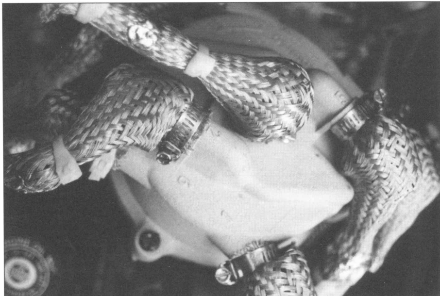
Fig 1—Braid installed over spark-plug wires at distributor.
