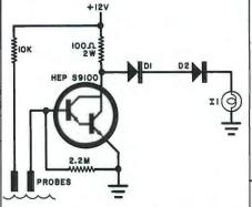
reservoir, leaving tips about 1 inch (2.5 cm) above the bottom. Install indicator *I*1 (which can be a 53 pilot bulb, a Sonalert or a buzzer) at a convenient viewing angle. When the fluid level drops below the probe tips, the lamp will light. Diodes *D*1 and *D*2 can be common 1-A power supply rectifiers. The alarm will work with water and most detergent solutions.
