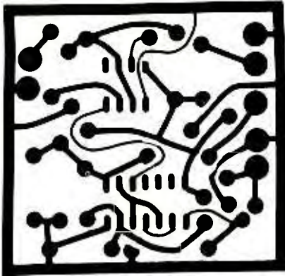
Fig. 3. Actual-size etching-and-drilling guide for printed-circuit board fabrication.
