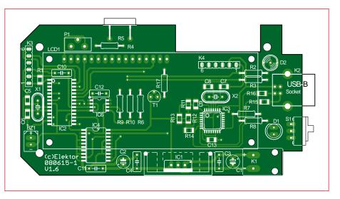
Figure 6. Board component layout.
