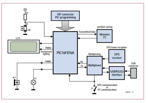
Figure 1. Block diagram of POI warning device.
