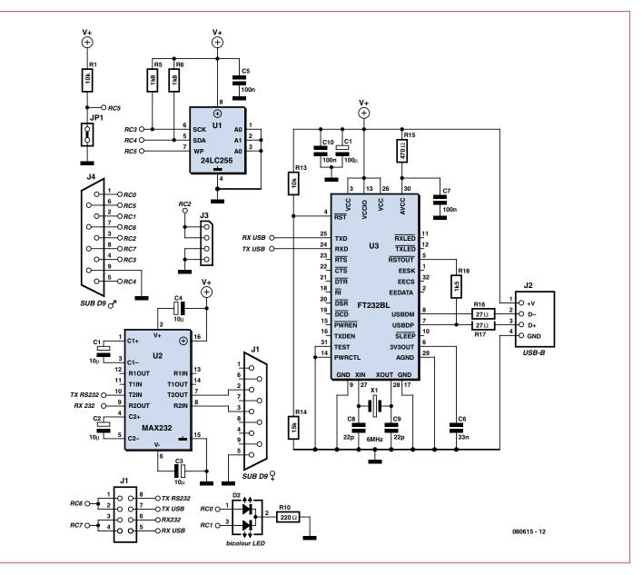
Figure 2. Circuit diagram of the home-made E-block. The serial data input is selected manually by the position of the jumpers on J1.
