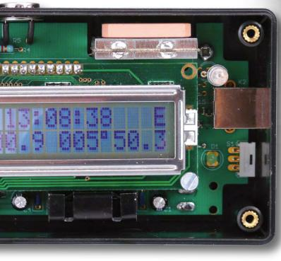
sounds, the bi-colour LED lights up red and steady, and the LCD displays a warning message. The MMI has one little unexpected extra: automatic backlighting that adjusts itself to the ambient light level.
