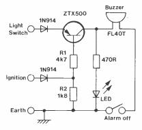
If the ignition is switched on, the transistor base is taken high, it no longer conducts, and the alarm ceases.
