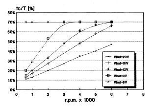
Fig. 9 - Conduction angle versus r.p.m.
