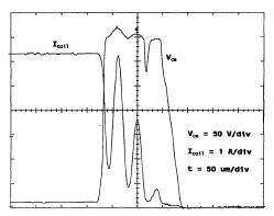
Fig. 8 - Turn-off with open gap.
