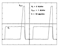
Fig. 4 - Duty-cycle = 70%; frequency = 20 Hz.
