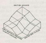
Fig. 7. Ignition or engine map using the distributor system.
