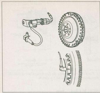
Fig. 6. Flywheel reluctor sensor. This comprises a magnet with a increase in dwell projecting pole piece and a reluctor disk on the flywheel. period compared
