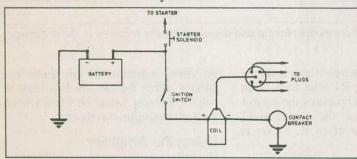
Fig. 1b. Conventional system with an in-circuit current-limiting bal- rate of switch-off lastresistor.
