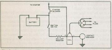
Fig. 1a. A conventional breaker ignition system.
