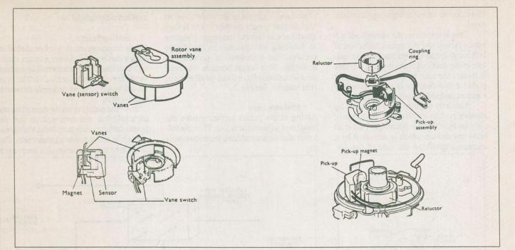
Fig. 4. Hall effect arrangement. (a) Vane switch (or sensor) and Fig. 5. Early distributor reluctor system arrangement. (a) Releuctor rotor vane. (b) Interaction of rotor vane and sensor. and pickup, (b) Reluctor tooth and pickup alignment.
