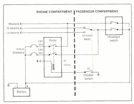
Fig. 7. Complete schematic diagram of the Automatic Headlights Circuit. It consists entirely of a 12-volt dc relay, two 20-ampere self-resetting circuit breakers, a single-pole, single-throw toggle switch and No. 14 insulated stranded wire.
