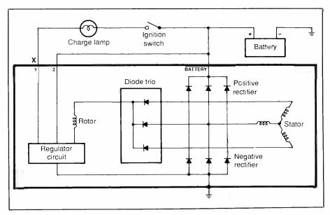
Fig. 1. Details of 1981 Chevette charging circuit.
