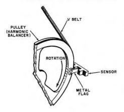
Fig. 3. Metal flag, % in. by % in. is attached to rim of harmonic balancer pulley to pass through slot in sensor interrupting light beam.
