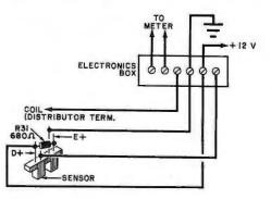
Fig. 5. External connections to the ignition monitor.
