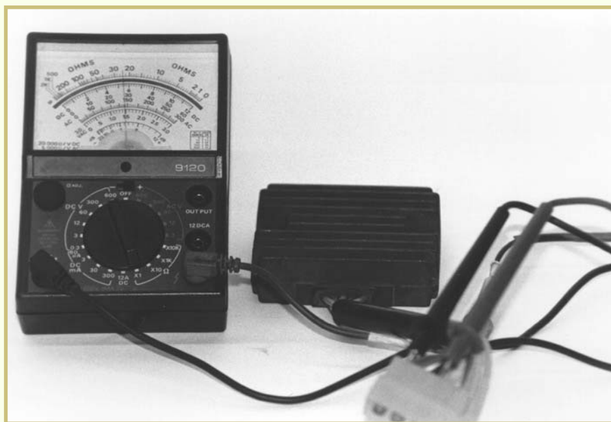
FIGURE 27 —Testing a rectifier in the forward bias should give a reading of 5–40 ohms.
