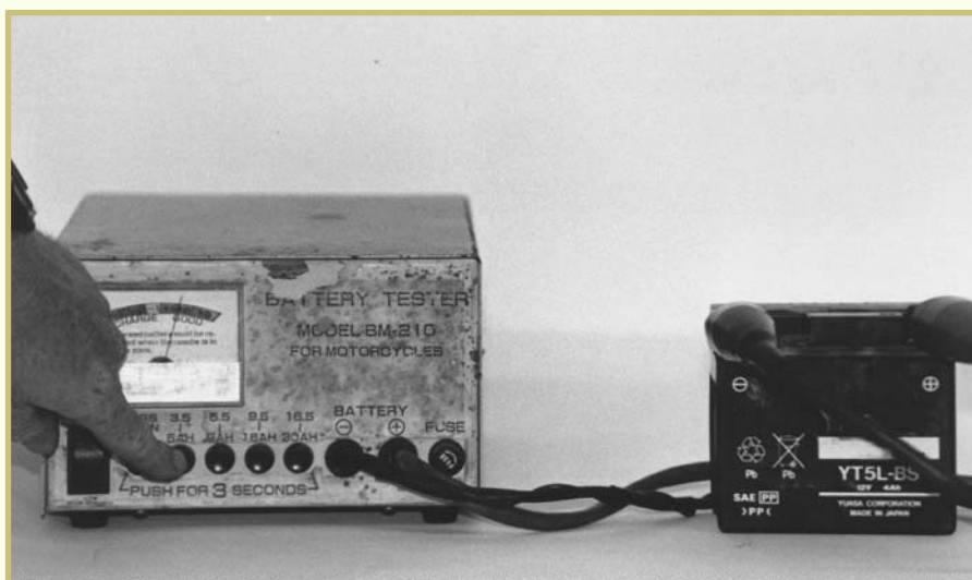
FIGURE 25 —The technician is checking the battery under a predetermined load by pushing the button on the tester. This battery is satisfactory because the needle is in the “good” portion of the meter face.
