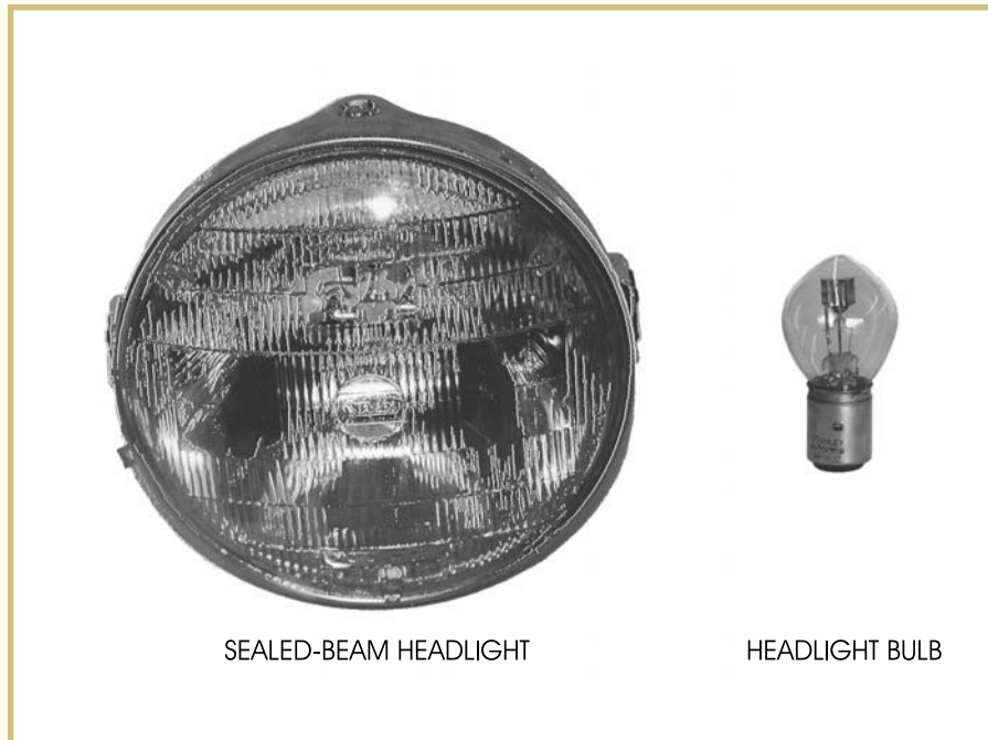
FIGURE 33 —This picture shows a headlight and a replaceable headlight bulb.
