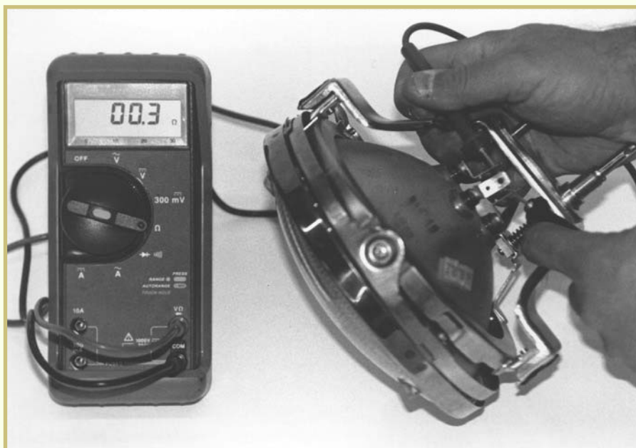
FIGURE 32 —A technician is checking a headlight by testing for continuity.
