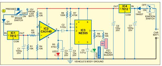
low to switch off the red LED. The low output of IC2 gives a short negative pulse to the monostable through C2 to trigger it. This activates the buzzer and LED2 to indicate that the brake system is working. When there is pressure drop in the brake system due
