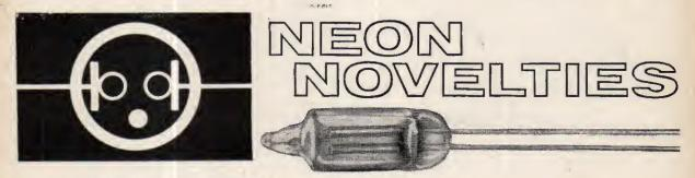
THIS is the first of a series of short articles illustrating some of the many uses of neon lamps. The neons employed are all miniature wire-ended types as shown above. Two examples which are ideally suited to these applications are those supplied by Radiospares (striking voltage 65 volts), and the Hivac type 3L general purpose neons. The latter type requires a striking voltage of 80 volts and maintaining voltage of 60 volts.
