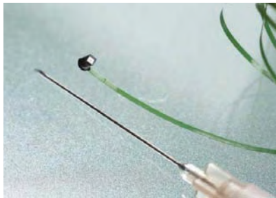
Figure 4 The Fraunhofer Institute expects to bring to market a camera as small as a grain of salt, which could replace side-view mirrors, reducing airflow drag.
