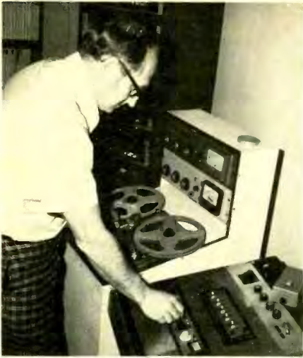
Garber checks a microphone volume level for proper setting during a recording session. The row of switches above the mixing controls operate equalizers which are used to enhance or diminish certain frequency ranges during a recording session or in making a copy or dub taping. A professional Crown stereo tape recorder is at Garbers right.
