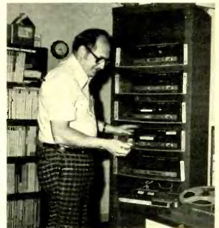
Garber stands beside his custom designed cassette duplication equipment to check the volume level for proper range. Asbury Records can duplicate cassettes at the rate of six at a time. The large bookcase stores master tape recordings.
