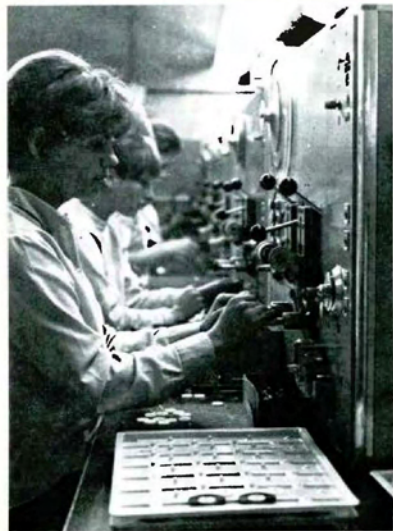
Fig. 4. These tailoring machines take reels of duplicated albums and wind them onto individual hubs that will fit the cassettes. A sensing device activates a cutting mechanism that separates the individual album hubs of tape.
