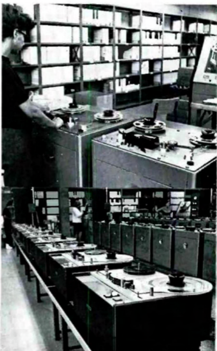
Fig. 1. These two Ampex 3300 mastering units, using 1/2 inch tape, feed a line of ten cassette duplicators. Continuous tape duplicating is possible with the two masters operating alternately. All illustrations have been made at the Ampex facility in Elk Grove Village, Illinois.
