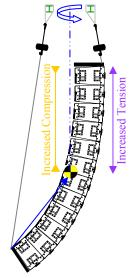
The total accumulated load occurring behind the cluster's center of gravity is distributed back through the array; and can manifest itself as torsion on the enclosures, the suspension grid, and eventually the structure.
