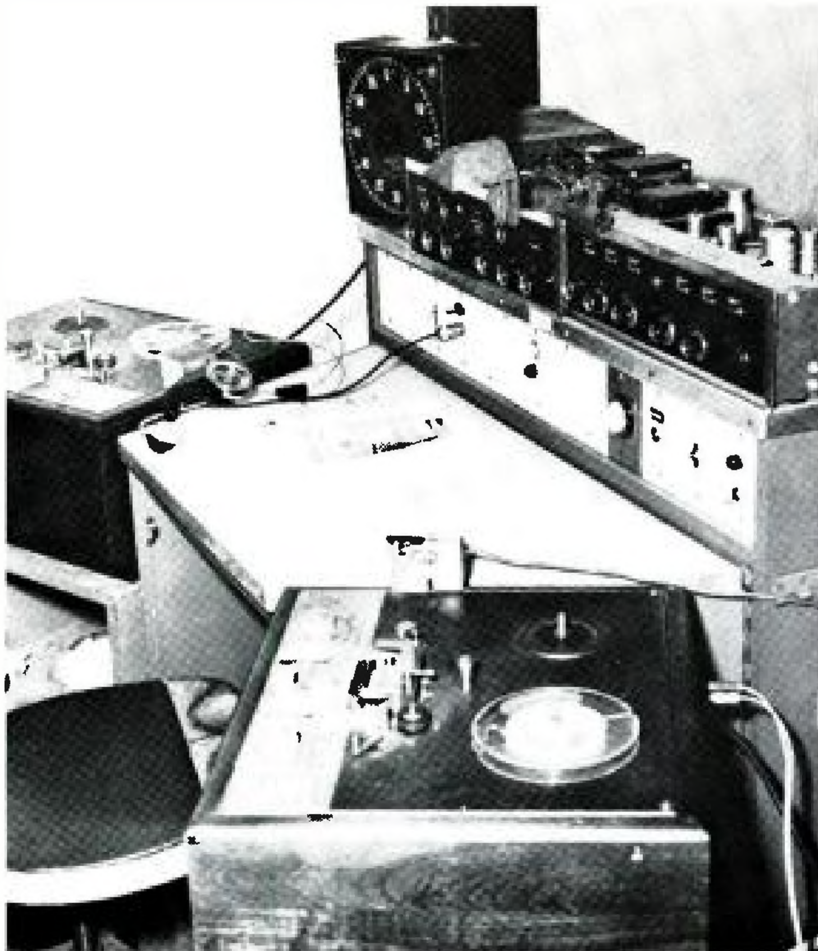
Fig. 3. A view of the sound console at The Players Club. The telephone headset connects with the lighting panel backstage. The Gralab photography timer is used to backtime music for synchronized-with-action endings. The two recorders are Ampex 936 units. The integrated stereo amplifier (upper left) and the stereo preamplifier (to its right) are both Scottkits.
