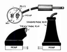
Fig. 1—Headphone makes telephone pickup.
