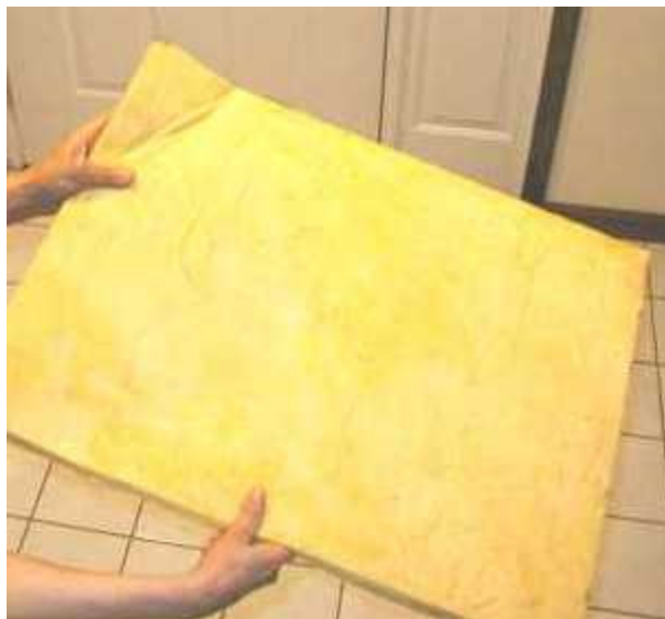
703 "rigid" fiberglass is not really very rigid.
