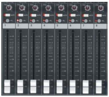
Pan-Faders.jpg A mixing console typically gives its best signal-to-noise performance with the input faders at 0. This is also known as 'unity' and is often marked by a heavier
