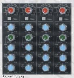
To set up the console, begin by turning down all the input gain (also known as trim or input level or input sensitivity) controls and set the equalizer level controls to the 12 o'clock position.
