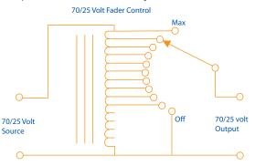
These controls will reduce the volume to the systems that they feed, still at 70 (25)-V. Although not usually done, use of series/parallel circuits can still be used on the 8-ohm output side of the transformer to limit the number of transformers used in low power situations.
