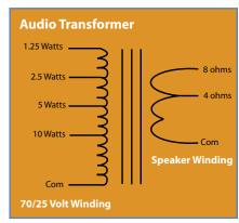
The 70(25)-V line from the amplifier is applied to the input of the transformer. The input selected is based on the maximum power needed from the speaker. Each speaker location comes from this same 70(25) volt line source (in parallel). The sum of the power setting of all transformers used should be less than the maximum power of the amplifier.
