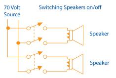
If designed properly, switching speakers on and off should not affect the levels in other speaker locations.
