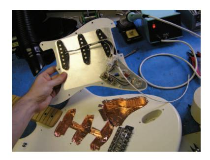
A good option is to add a copper or foil shield inside the pickup and electronics cavity of the guitar. Copper shielding with an adhesive on one side works best. Be careful to push the copper tight against the wood to ensure you do not cause any electrical shorts. You should then shield the pickguard if you have a Strat type guitar. All of the shields should then be tied together (soldered) to create a uniform shell around the electronics. This is then grounded at the guitar jack.
