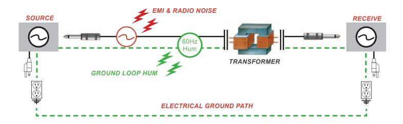
A transformer is basically a magnetic bridge. In other words, current goes into the primary coil and is 'transformed' into a magnetic field. The magnetic field is then guided to a secondary coil where signal is produced. Because the input and output are not connected - they are magnetically bridged - any DC noise that may be problematic is eliminated. This is because transformers only pass alternating current (AC) not direct current (DC).
