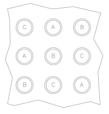
Figure 5. Noise Masking Ceiling Array
