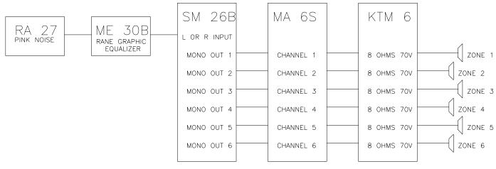
Figure 4. Basic Noise Masking System Example
