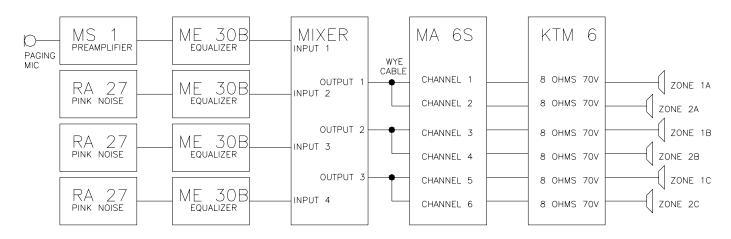
Figure 5. Multiple Array Noise Masking System Example
