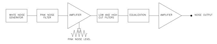
Figure 3. Typical Noise Maksing Generator
