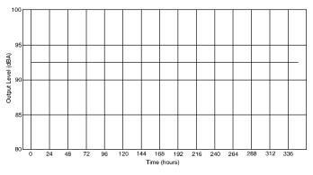
Figure 2. RA 27 Pink Noise Level Stability with Time Noise Masking-2
