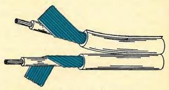
Fig. 2. Stereo cable with separately wrapped shields.
