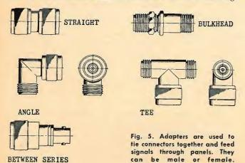
adapters. Also, when calling out a between-series adapter, it is necessary to indicate the specific series involved, such as an adapter with a BNC female end and a series N male end.
