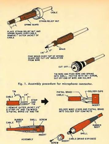
Fig. 2. When assembling multi-contact connectors, the insulation should butt the pins, and the conductors and pigtails be pretinned before placing in the solder cups.
