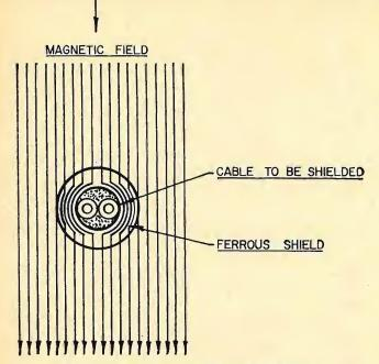
Fig. 4. Ferrous materials repel external lines of flux.
