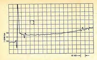
Fig. 5. Impedance changes along the length of a cable.
