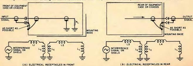
Fig. 4. Cable shield bonding for chassis connectors (A) when receptacles are on front panel, and (B) are on rear of chassis.
