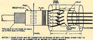
STRUCTURE OR CONNECTED BY MEANS OF EAREO WASHER 2. HALO IS 1/4" TO 1/2" WIDE
