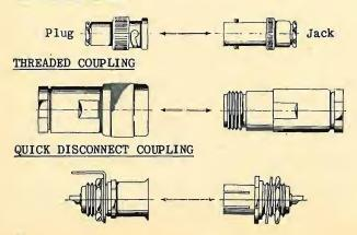
by the size of cable for which they are designed, that is, they can be classified as small, medium, or large. Cables whose dimensions, for example, exceed  $\frac{1}{4}$ -in diameter are generally well suited to connectors of the UHF and type N style; below  $\frac{1}{4}$  in, BNC and TNC are popular. For tiny miniature cables, the subminiature connector types such as the Amphenol 27 series (MIL-C-22557) or new SMA microwave subminiatures should be used. See Table 1.
