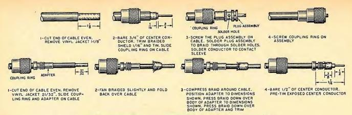
Fig. 2. The assembly method covering the 83-1SP plug and adapter. See text for details.
