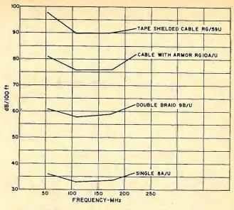
Fig. 3 Relative shielding efficiences for various cables.
