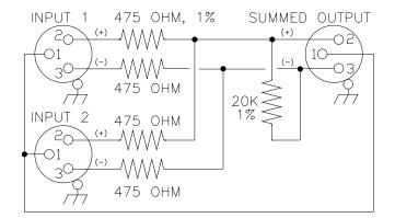
Figure 2. Balanced summing box using XLR connectors
