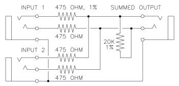
Figure 3. Balanced summing box using 1/4" TRS connectors
