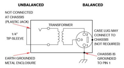
Figure 2. Transformer Isolation
