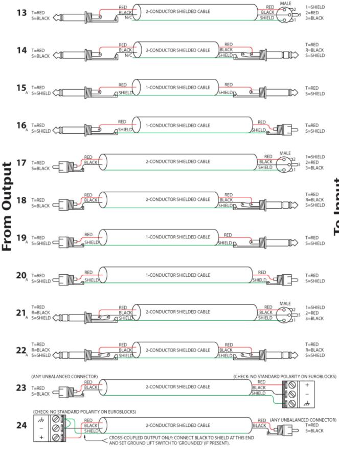
Figure 4. Interconnect chart for locating correct cable assemblies.
