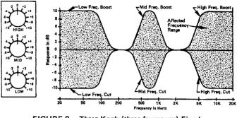
FIGURE 9 – Three Knob (three frequency) Fixed Frequency Equalizer
