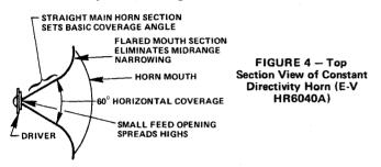
Most conventional horns have a long tapered "throat" that has a rather large opening by the time it reaches the main section of the horn. This means that the highest frequencies are *not* spread enough to be controlled by the main section and tend, instead, to beam straight ahead (the higher the frequency, the more straight ahead). See Figure 5 for a horn whose large throat opening cannot spread the highs.
