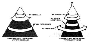
FIGURE 1 — Horizontal (Side-to-Side) Coverage Angle Comparison, Constant Directivity and Coventional Radial Horns
