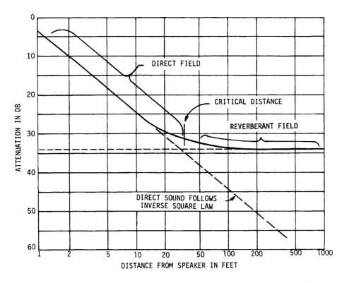
FIGURE 6 – Attenuation with Increasing Distance in Typical Large Room
