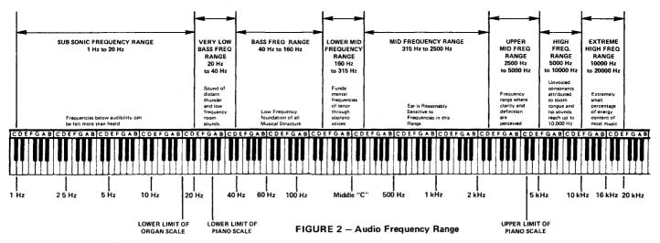
to provide a visual aid. It was mentioned earlier that the range of human hearing is 20 Hz to 20 kHz. This would be the frequency range for a person with very good hearing. Most types of professional audio equipment will have a specified frequency response of 20 Hz to 20 kHz. For our purposes we will now investigate the frequency range from 1 Hz to 20 kHz.
