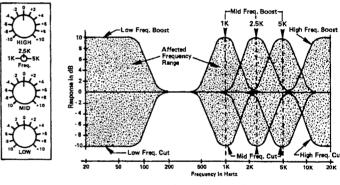
FIGURE 10 - Three Knob (five frequency) Equalizer with Switchable Mid-Range
