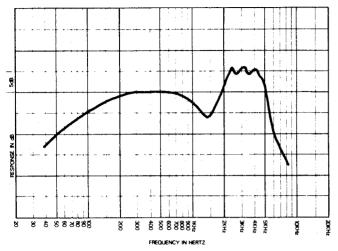
FIGURE 3 - Small Coil (1.75 in.) 12 in. Guitar Speaker
