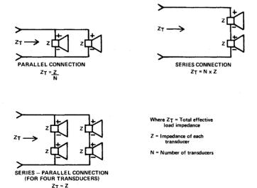
FIGURE 7 – Loudspeaker Connections
