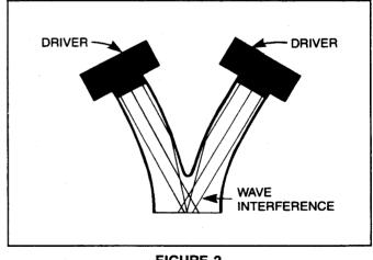
FIGURE 2 "Y" Manifold Showing Ray Interferences
