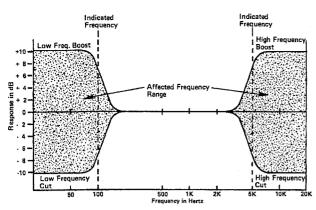
FIGURE 3 - Shelving Equalization Curve
