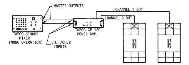
FIGURE 12 - Block Diagram for Medium Size Room, Setup Number 1
