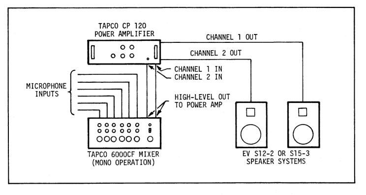
FIGURE 10 - Block Diagram for System Shown in Figures 8 and 9
