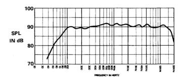
FIGURE 7 – Axial Frequency Response (Bandwidth)
