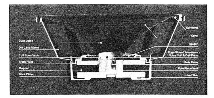
FIGURE 7 - EVM Cutaway
