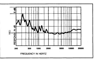
FIGURE 9 — Impedance Altec 288-8K Driver on EV HP9040 Horn
