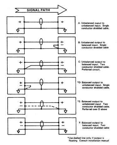
FIGURE 5 - Interconnecting Circuits
