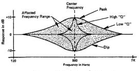
FIGURE 5 - "Q" of a Peak/Dip Equalizer
