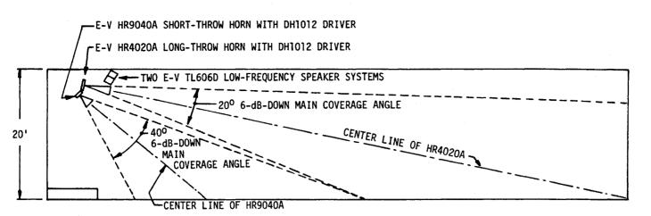
FIGURE 21 - Elevation View of Large Size Room, Permanent Installation
