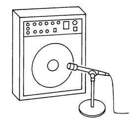
FIGURE 5 – Amplified Guitar Microphone Placement
