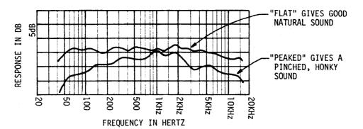
FIGURE 1 – Axial Frequency Response
