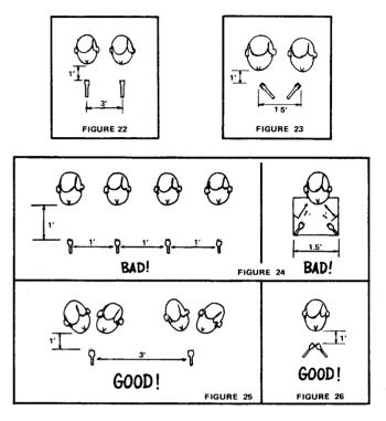
When two microphones must be used close together, multiple interference can be avoided by placing the heads directly together. (See Figure 26)
