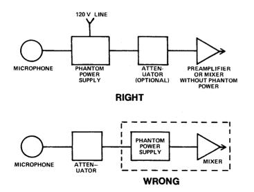
FIGURE 1 — Phantom Powering
