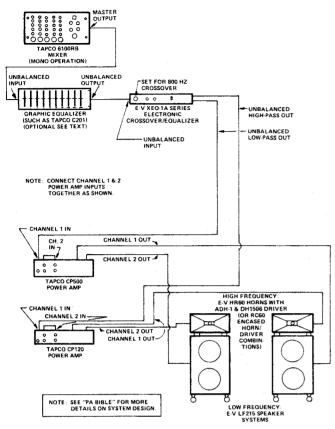
FIGURE 11 – Block Diagram of Typical Two-Way Component System
