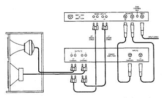
FIGURE 1 — A block diagram of a controlled speaker system.
