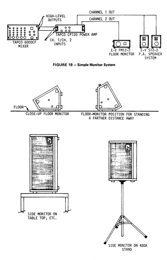
FIGURE 20 – Various Possible Placements of FM12-2 and FM12-3 Floor Monitors
