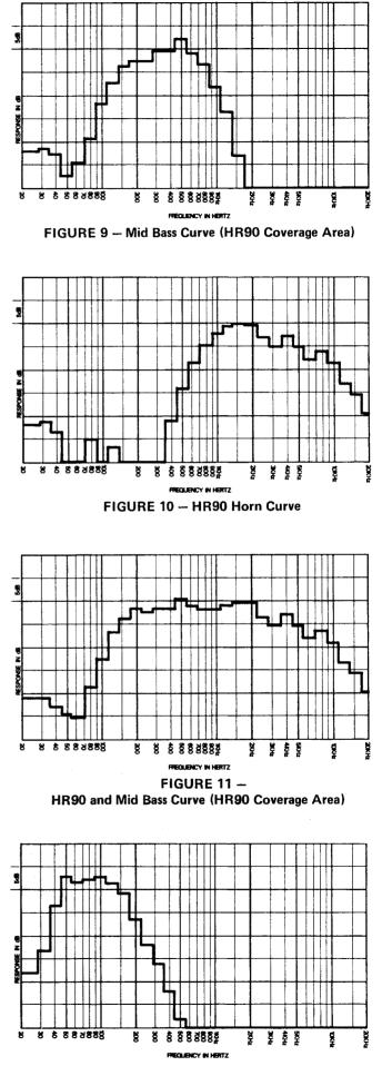
FIGURE 12 – Sub-woofer Curve (HR90 Coverage Area)
