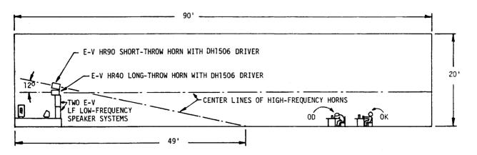
FIGURE 16 – Elevation View of Large Size Room
