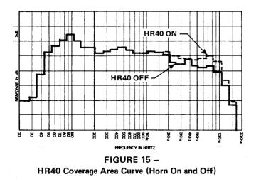
Switching on the long-throw horn brought the sound clearly into focus, getting a quality strikingly similar to that observed from a position in the pattern of the short-throw horn.
