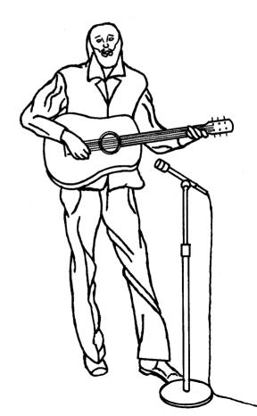
FIGURE 7 - Acoustic Guitar Microphone Placement
