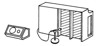
FIGURE 6 - Piano Microphone Placement
