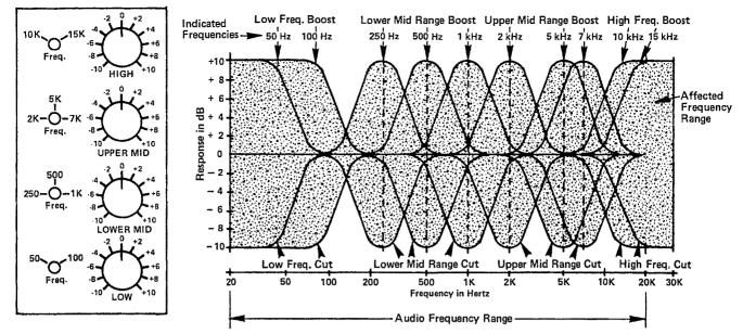
FIGURE 11 - Four Knob (ten frequency) Selectable Frequency Equalizer
