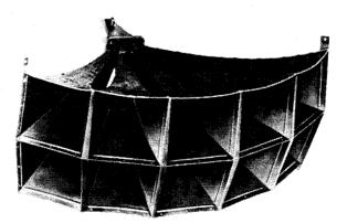
FIGURE 3 - Multicell Horn
