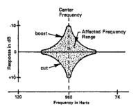
FIGURE 4 - Peak/Dip Equalization Curve
