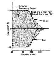
FIGURE 6 - "Q" or Slope of a Shelving Equalizer
