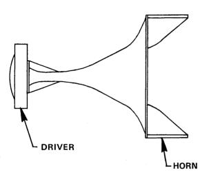
FIGURE 1 – Simple Driver and Horn View
