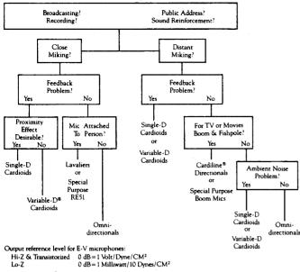
FIGURE 19 - Microphone Application/Recommendation Chart
