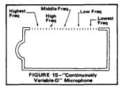
In addition to reduction of the Single-D's proximity effect, Variable-D and Continuously Variable-D cardioids have reduced breath popping and shock sensitivity. Thus, the popularity of the Variable-D microphone is due to its combining of the omnidirectional's clarity and inherent pop and shock resistance with the cardioid's feedback reduction and working distance advantages.
