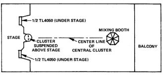
FIGURE 7 – Horizontal Positioning
