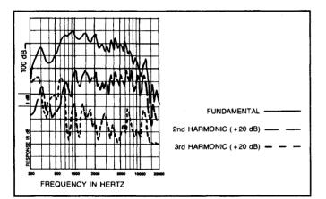
FIGURE 6 — Response & Distortion; Altec 288-8K Driver on Altec MR-94 Horn (1 watt, 10 feet)
