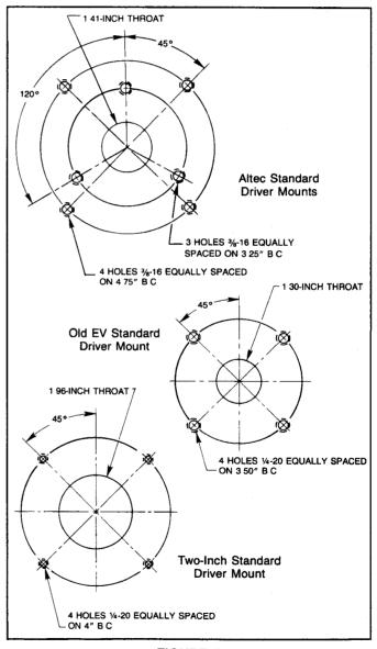
FIGURE 5 Large-Format Throat Configuration
