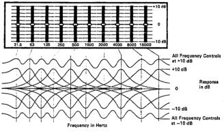
FIGURE 12 - One Octave Graphic Equalizer
