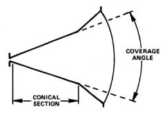
FIGURE 8 - Conical Section of Horn
