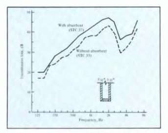
Figure 1. Actual measurements showing improvement of transmission loss of double glazed windows by covering the edges of the interpane activity with sound absorbing material. A gain of 4 STC points is attributable to the absorbent. In this case, 5/32-inch (4mm) glass is used. Improvement of TL due to absorbent is greater with thin than with heavier glass. (Adapted, with permission, from A. Cops et al.)
