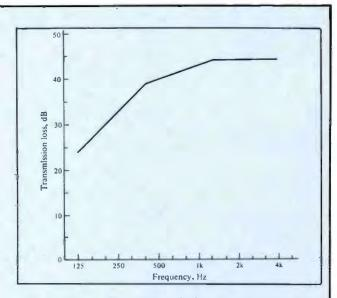
Figure 1. The standard STC contour.
