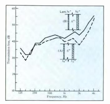
Figure 3. Laminated glass offers less stiffness than comparable solid glass: (A) Normal double glazed window of 1/4-inch and 1/2-inch glass sheets spaced 6 inches; (B) the same window except the 1/4-inch solid sheet has been replaced by two 1/8-inch sheets laminated with 0.045 inch plastic. The window with the laminated sheet shows the greater transmission loss. (Libby Owens Ford, Ref. 3.)
