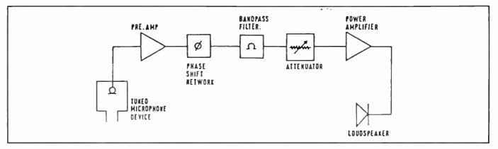
Figure 1. Block diagram of the basic system channel.
