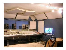
Symmetry is equally important, so center your desk and speakers left-right in the room. Placing the mix position in the front part of the room also helps the low end response. The ideal speaker height is with the tweeters at ear level, because the flattest response is on-axis. I prefer speakers to be level, not angled down to your ears. Otherwise, as you move forward and back slightly the high frequency response changes. The article <u>How To Setup a Listening Room</u> explains more.
