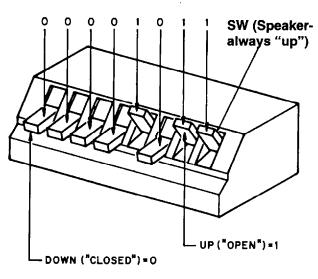
Important: The rightmost key, marked "SW" on the circuit board, must always be in the up ("1") position. This indicates that the board is controlling speakers, the only option for staff stations in a 2524 system.
