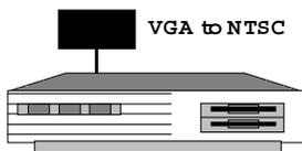
RANMENU uses an IBM compatible PC to generate and display classroom TV menus for the RANGER system. A PC running RANMENU software interprets live serial data fed from a RAN232 Serial Control Card housed in the RANCC16 Control Card Cage. The data is formatted and sent to the computer VGA video output where it is converted to a composite NTSC signal via a VGA/NTSC scan converter. The video output is then
