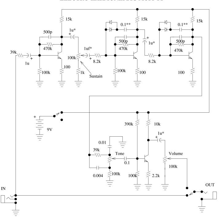
The EH Big Muff Pi would probably be improved by modern input-jack power switching and a DPDT bypass switch. This is the original schematic. The diode and transistor types are unknown. Probably any high gain NPN and 1N914s work. Coupling caps marked by a \* have been reported to sound better if changed to 0.1uf as have the \*\* marked ones if changed to 1.0uf. The original transistors were marked SPT 87-103, and the original diodes were marked 525GY or 523GY (hard to read).
