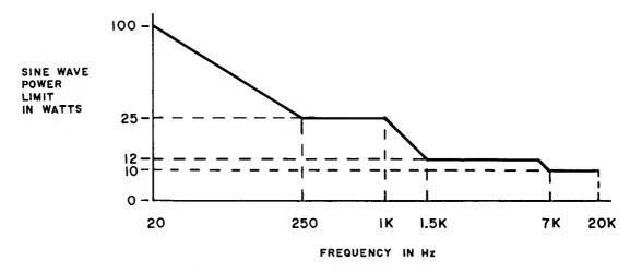
Avoid operating the speaker system with sustained sine wave signals at power levels greater than the indicated limits. Permanent damage may result.
