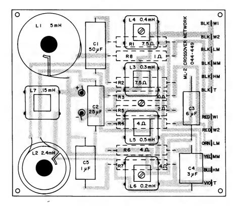
TWO DIFFERENT CIRCUIT BOARDS HAVE BEEN USED. THE SCHEMATIC IS THE SAME FOR BOTH.
