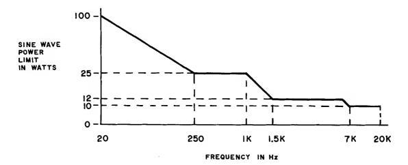
Avoid operating the speaker system with sustained sine wave signals at power levels greater than the indicated limits. Permanent damage may result.
