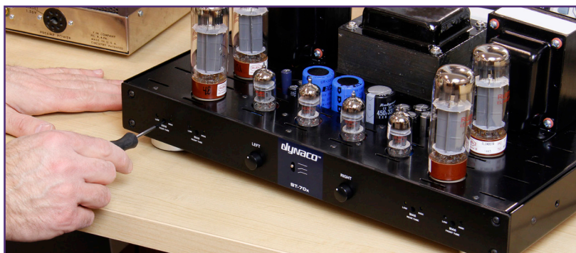
Photo 8: Adjusting the bias on the new Dynaco ST-70 Series 3.
