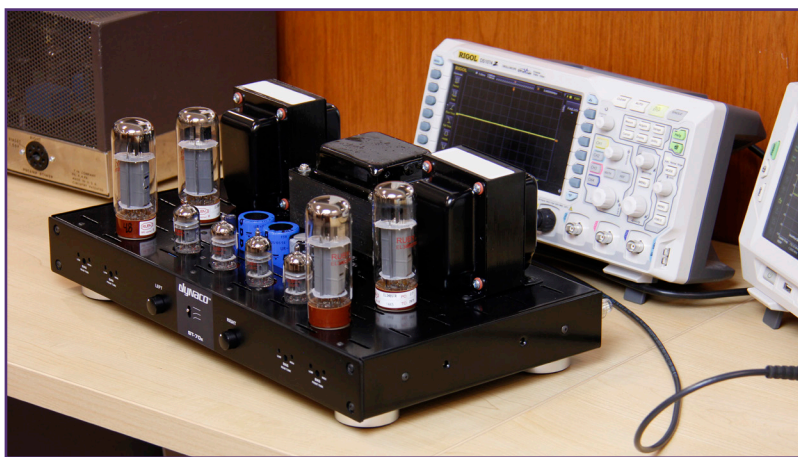
Photo 1: The new Dynaco ST-70 Series 3 tube amplifier intends to be an updated version, compliant with today’s demanding global regulatory safety requirements.
