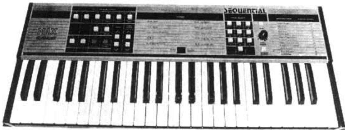
Figure 20.13 A MIDI synthesizer capable of using the multi-timbral Mono Mode – the SCI Max.
