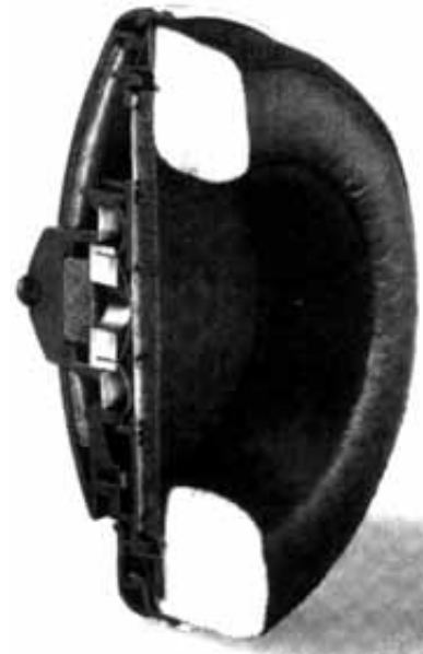
Figure 17.4 Cut-away view of a Sennheiser headphone earpiece showing the diaphragm, magnets and acoustic damping materials.
