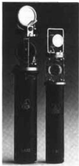
Figure 2.24 Examples of stereo microphone design allowing the mutual angle between the two capsules to be adjusted by rotating the upper capsule (AKG C422 and C34).
