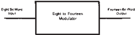
Figure 5.21 The eight to fourteen modulator.
