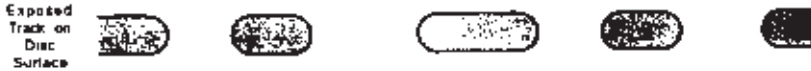
Figure 5.18 The sequence of dashes created where the laser beam has been switched on.
