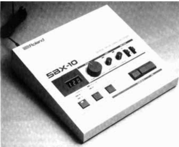
Figure 20.10 A MIDI-compatible synchronizer – the Roland SBX-10.
