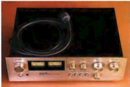
This secondhand amplifier – bought for just $8.00 – was the guinea pig for much of the testing described here. Using just simple tools and techniques, its power output, frequency response and signal-to-noise ratio were all measured, along with the response of its tone controls.
