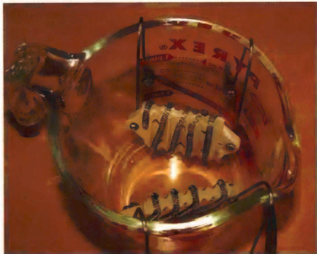
The amplifier test load is formed by two slightly modified electric jug elements suspended in a jug of cooling water. This load can sink very large power outputs – if the water starts getting hot, simply swap it for some cold water.
