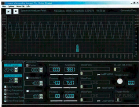
Fig.2: this audio frequency generator software is available for a 30-day free trial period via a web download. Just about any frequency generator software is suitable for the amplifier testing procedure described in this article.
