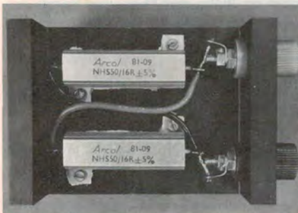
ETI-155b 8 ohm, 100 W dummy load using non-inductive resistors.
