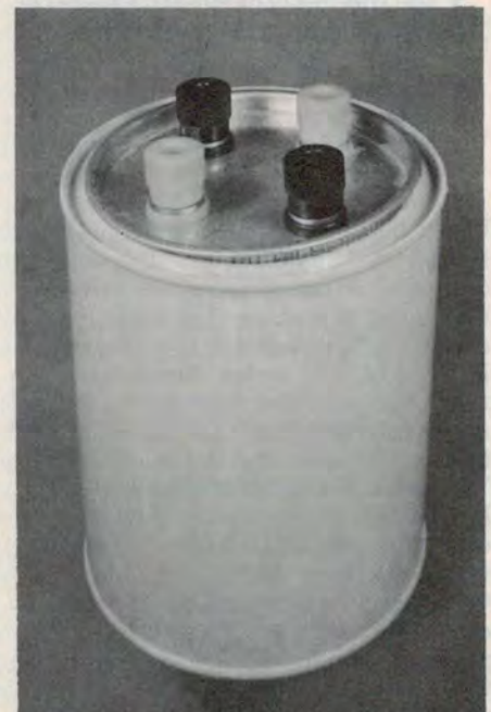
ETI-155a 4, 8 or 16 ohm dummy load (50 or 100 W) using 98 390 ohm 1 W resistors.
