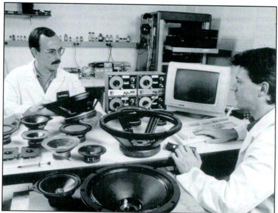
Figure 1. Audio engineers run a vast array of speaker tests, free to customers. Damping, heat transfer, impedance and ferrofluid compatibility are checked.
