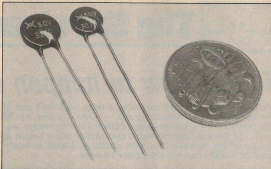
Pictured are the two Polyswitch Protectors which will be initially available from parts stockists. They are the RDE 050 and RDE 115A.
